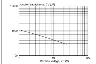
Typical junction capacitance;  $C_d = f(V_R)$ ; f = 1 MHz;  $T_j = 25^{\circ}\text{C}$  to  $125^{\circ}\text{C}$ . Fig.5.
