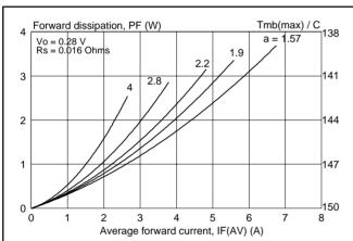
Fig.2. Maximum forward dissipation  $P_F = f(I_{F(AV)})$ ; sinusoidal current waveform where a = f(AV) $factor = I_{F(RMS)} / I_{F(AV)}$ .
